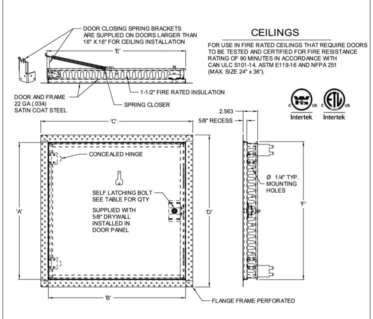
STANDARD FEATURES: UNIVERSAL SELF LATCHING BOLT- OPERATED BY FLUSH KEY, WITH INSIDE TURN RELEASE SATIN COAT STEEL, MILL FINISH
