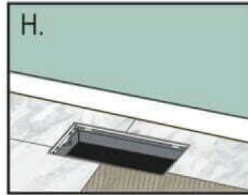
H. Repeat the process until frame is completely enclosed with your tiles.
